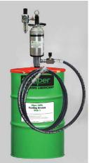
The new Viper Mk II kit includes an upgraded lubricant pump, built specifically for the Viper WRL. Two pump options are available the standard unit delivers 4.5kg/min. while the optional High volume unit delivered 13kg/min for fast lubrication of large diameter ropes, for further reduced down time. Both pumps are supplied in 190kg drum size with the option of 20kg Drum size available with the standard pump.
